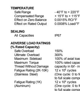
100% of axial load capacity 100% rated capacity lbf-in capacity in lbf - in 12 x 10<sup>6</sup> cycles (One cycle: 0 to full scale tension to full scale compression) 12 x 10<sup>6</sup> cycles (One cycle: 0 to full scale tension to full scale compression)
